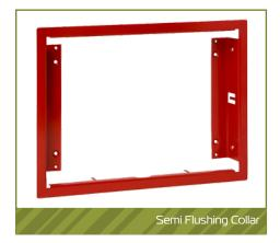
The eView semi flushing collar allows the eVIEW annunciator to easily be recess mounted. Flushing collars provides placement tabs that fold behind dry wall. Traditional screw mounting is available by 2 openings in each of the vertical frames. Conduit entry is not blocked by collar.
